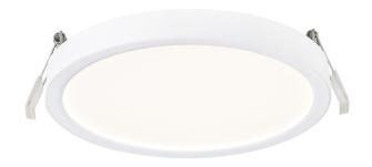
Height (cm): 2.5 Projection (cm): 2.5 Diameter (cm): 23.4 Hole diameter (cm): 20 Mounting height (cm): 4.5
